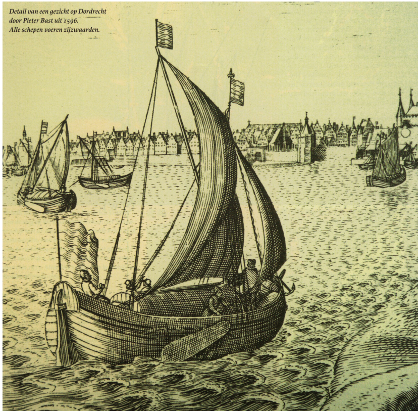
Illustration 1 Dutch ship with leeboard. Painting View on Dordrecht, by Pieter Bast 1596 (source: Rijksmuseum Amsterdam, http://hdl.handle.net/10934/RM0001.COLLECT.75856 )
